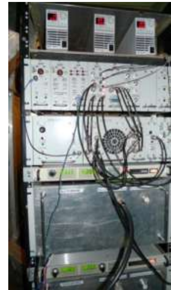
Ion source supply rack at 400 kV potential
