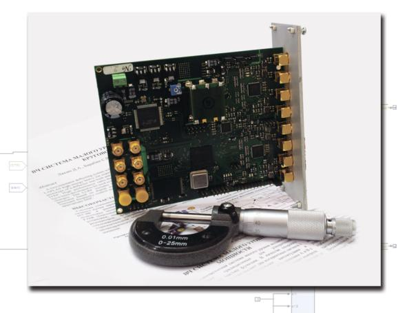
Four-channel RF signal measurement module combines on same board two ADCs with up to 100 samples per microsecond in IF mode.
