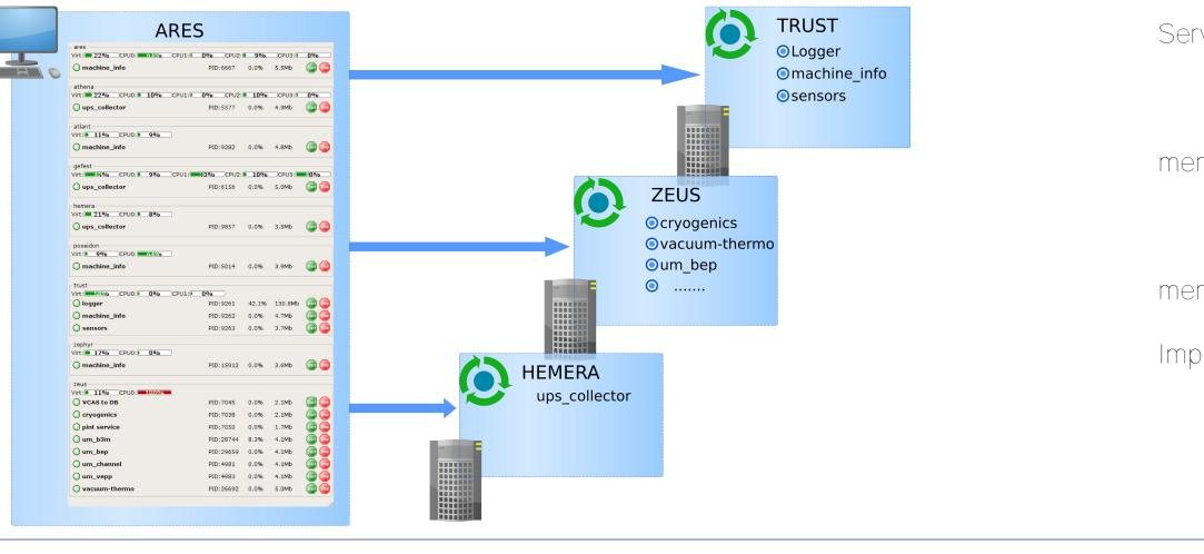
Service monitoring subsystem: •Service auto-start •Service info(status,CPU, memory) Manual service start/stop •Node workload (per CPU, memory) Implemetaion: •Supervisord •Custom made plugin (Pyhton)
