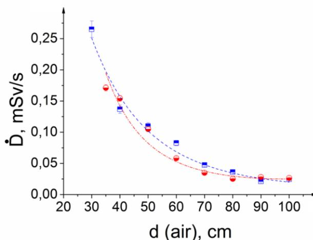
Fig. 2. The depth dose distribution in the air of the pulsed bremsstrahlung generated by betatron:  $\blacksquare$  – the solid thermoluminescent dosimeters DTL-02 measurement results;  $-\ - -$  the approximation results of the solid thermoluminescent dosimeters DTL-02 measurements;  $\bullet$  – the cylindrical ionization chamber type 30013 measurement results;  $-\ - -$  the approximation results of the cylindrical ionization chamber type 30013 measurements.
