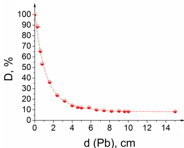
Fig. 3. The depth dose distribution in the lead of the pulsed bremsstrahlung generated by betatron; ● – the cylindrical ionization chamber type 30013 measurement results; - - - - the approximation results of the cylindrical ionization chamber type 30013 measurements.
