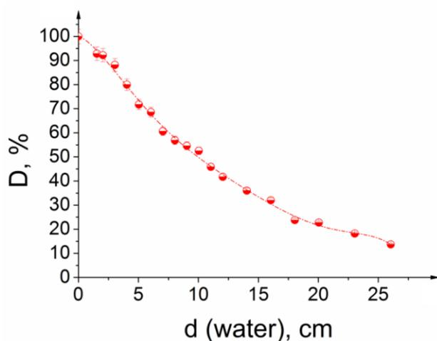
Fig. 4. The depth dose distribution in the water of the pulsed bremsstrahlung generated by betatron; ● – the cylindrical ionization chamber type 30013 measurement results; - - - - the approximation results of the cylindrical ionization chamber type 30013 measurements.
