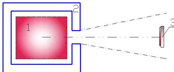
Fig. 1. The irradiation scheme: 1 – the portable betatron OB-4; 2 – the lead dome; 3 – the plane-parallel ionization chamber type 23342
