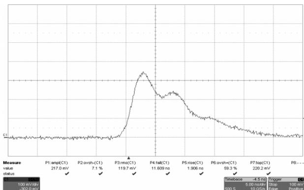
Figure 3: X-ray pulse shape of ARSA accelerator, registered with the aid of fiber-optic scintillation detector.
