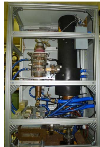
Fig. 2. Photo of the accelerator with the beam scanning system.
