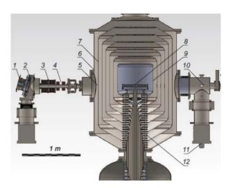
Figure 1: High-current vacuum insulation tandem accelerator. 1—H ion source, 2—diaphragm, 3 magnetic lenses, 4—corrector, 5—a temporary location of thebeam detector, 6—accelerator, 7—electrodes, 8 stripper, 9—high voltage electrode,10—high energy beam transport, 11—turbo molecular pumps, 12—insulator.
