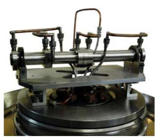
Figure 2: Ø16-mm stripping target placed on the feedthrough insulator.
