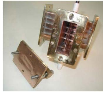
Figure 3: Packet of switches with mutual side arm.
