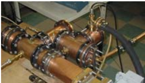
Figure 2: Microwave resonant compressor with the cascade switch based on two H-tees in side arms.
