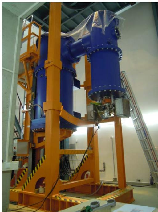
Figure 6: Assembled accelerator for tomography.
