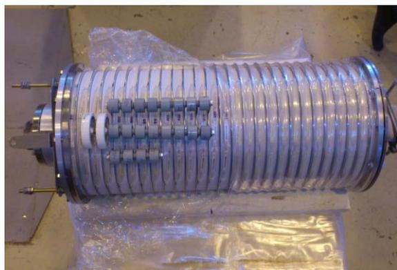
Figure 5: Modified accelerating tube.
