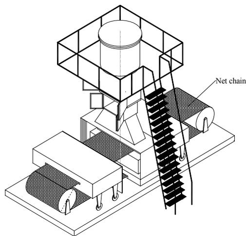
Figure1: 0.3 MeV\*100 mA accelerator for tire industries.
