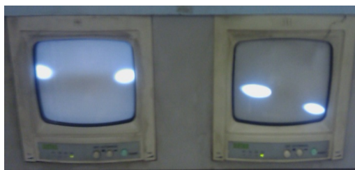
Figure 8. An image of colliding beams on screens of the SR monitors, i.e., a 1.1 mA electron (on the left) and 0.3 mA positron (on the right) beam; the voltage amplitude on the high-frequency separation plates is 6.5 kV ( E = 1.85 GeV), and two positions of the two-turn orbit are visible.
