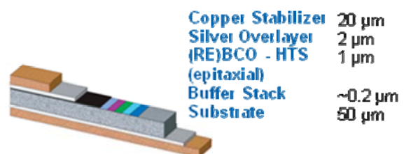
Figure 3: Structure of 2-G HTS tape (Re)BCO.
