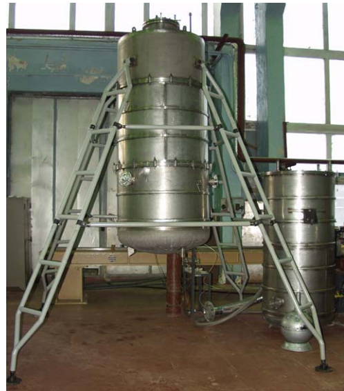
Figure 8: Cryogenic helium vacuum heat exchanger (10g/s helium flow, 300-2 K temperature range).
