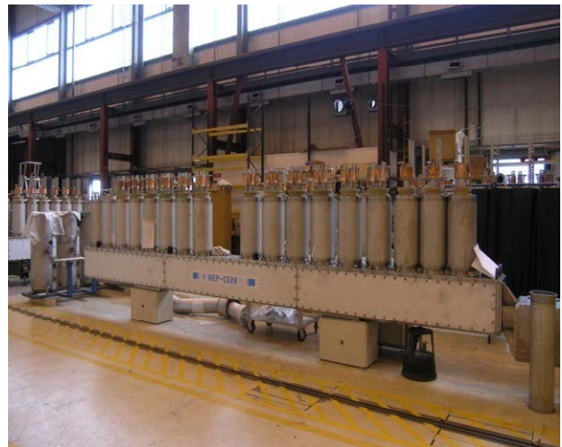
Figure 9: DFBA Cryogenic Electrical Feed Box for LHC.
