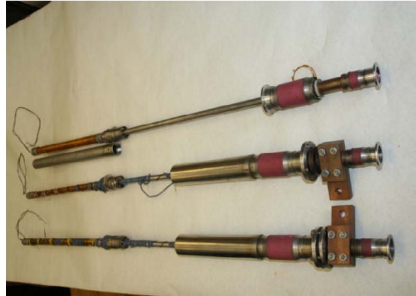
Figure 11: 600 A HTS current leads.
