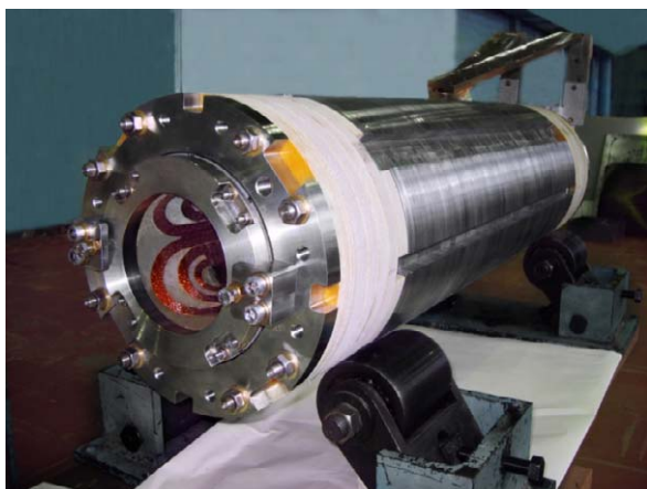
Figure 5: SIS300 fast cycling quadrupole prototype.
