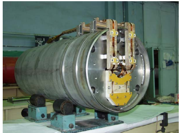
Figure 2: SIS300 high field fast cycling dipole model.
