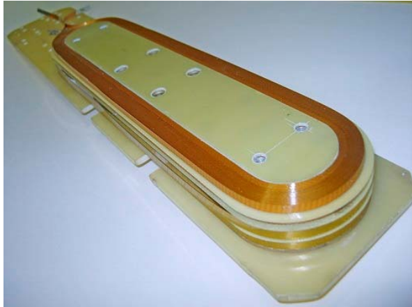
Figure 13: Four-layer racetrack coil from HTS-2G tape.
