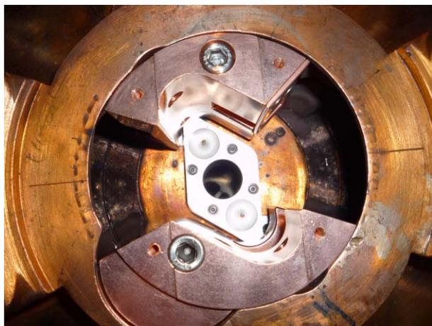
Figure 5: New central region of U200P cyclotron.
