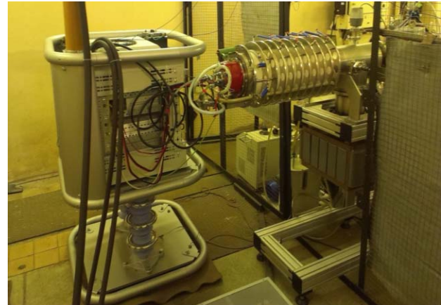
Figure 3: High-Voltage Structure of the Neutron Generator.
