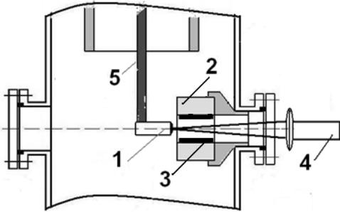
Figure 1: Laser-plasma diode. 1 – the anode with a laser TiD target; 2 – the hollow cylindrical cathode (NdFeB); 3 – place target, forming neutrons (DD reaction); 4 – laser radiation; 5 – vacuum electrical connector
