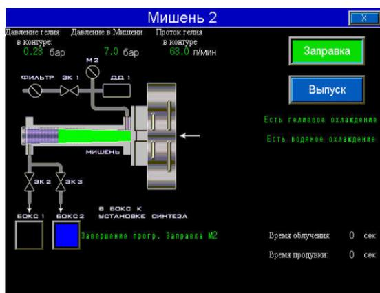
Figure 3: Window for operation with gas target.
