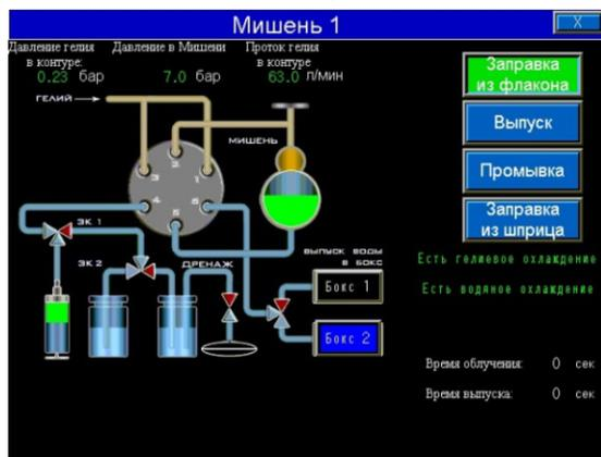
Figure 2: Window for operation with water target.
