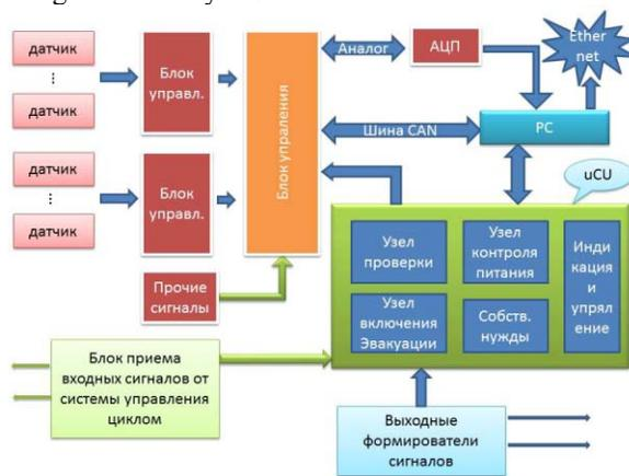
Figure 1: Block-diagram of the Nuclotron quench detection system.
