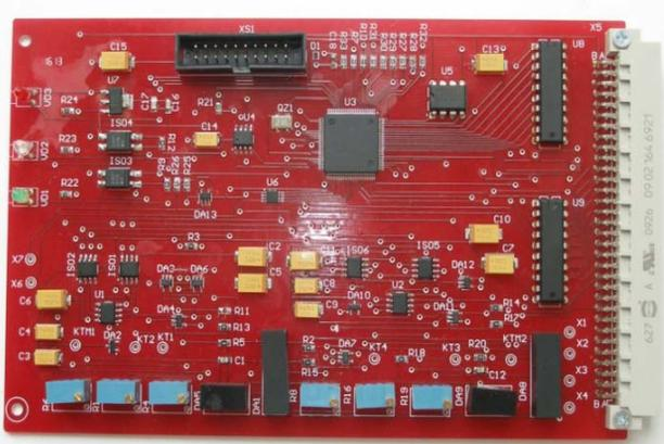
Figure 3: Printed circuit board of the quench detector
