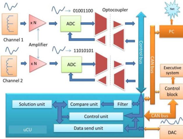
Figure 2: Block diagram of the universal quench detector.
