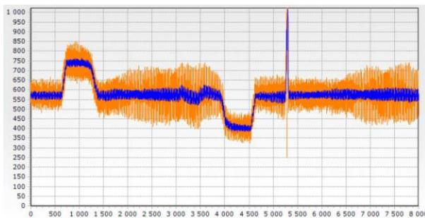
Figure 5: Signal from the quench detector at the filter input (yellow curve) and output (blue curve). Units of measure are the same as in indicated along the vertical axis; the entire scale corresponds to 3.3 V and the zero level is approximately 500. The time in hundreds of milliseconds is laid along the horizontal axis; i.e., the entire scale is 800 ms.
