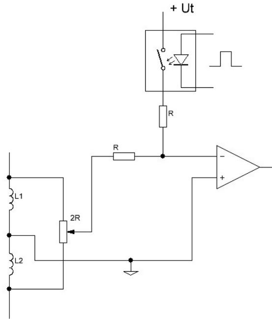
Figure 4: The system of checking circuits of communication and detector.
