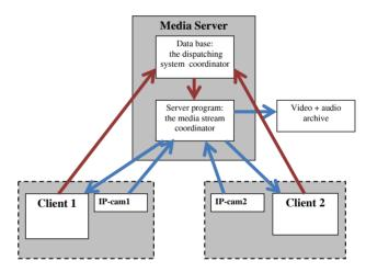
Figure 1: The scheme of the data flow (blue arrows) and the control flow (red arrows).
