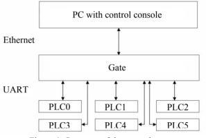
Figure 1: Structure of the control system.
