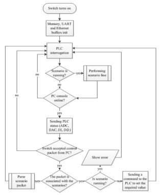
Figure 2: The basic algorithm of the switch.
