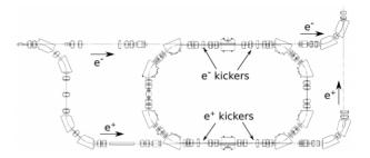
Figure 2: Damping ring kickers placement layout.
