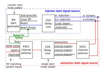
Figure 3: Kikers start signals sources layout.
