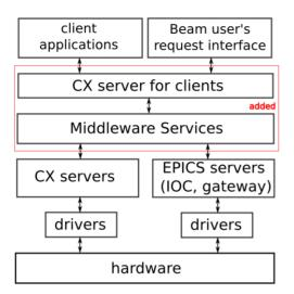
Figure 1: Injection complex software structure with middleware.
