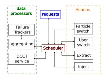
Figure 4: Injection/extraction control services.
