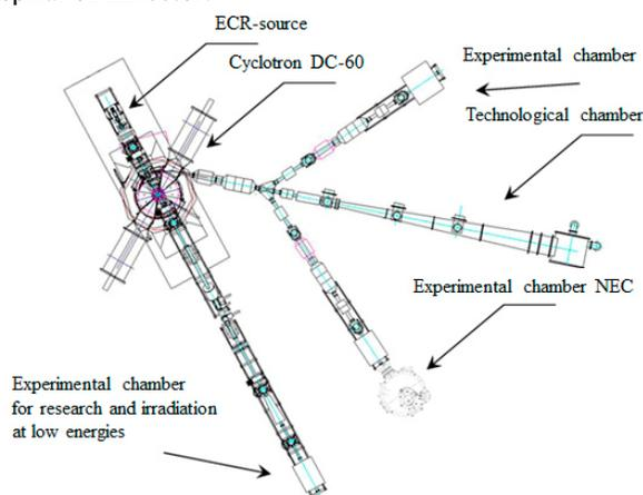
Figure 1: The scheme of the DC-60 accelerator complex.
