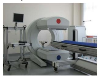
Figure 1: The «EFATOM» gamma-tomograph.
