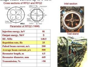
Figure 4: Design and parameters of RFQ-2
