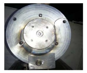
Figure 3: Target holder for TEM samples.
