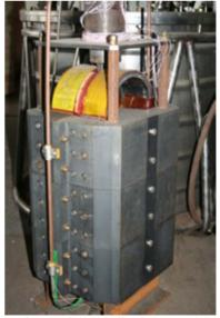
Figure 12: HTS dipole magnet.
