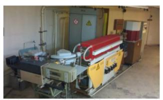
Fig. 2: Appearance of system of formation picoseconds pulses on accelerator UELV-10-10-T-1.
