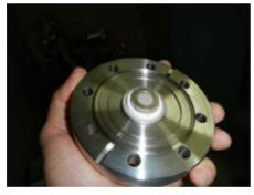
Figure 2: Flange welded grid-cathode assembly.
