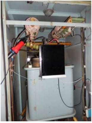
Figure 5: The modulator with semiconductor switche.
