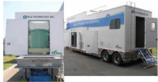
Figure 2: Mobile accelerator.
