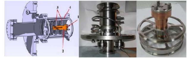
Figure 4: A) Target chamber construction: 1 – sample holder; 2 – copper ingot; 3 – stainless steel rings, 4 – water cooling system. B) Photo of system of sample holder C) Photo of copper ingot and stainless steel rings
