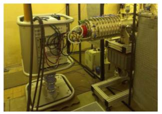
Figure 3: High-Voltage Structure of the Neutron Generator.
