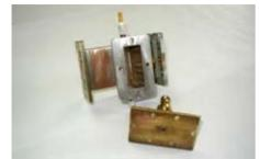
Figure 1: Interference switch on the basis of oversized rectangular waveguide.
