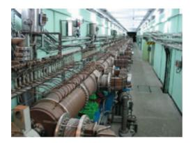
Figure 1: DAW accelerating structure in the INR linac.
