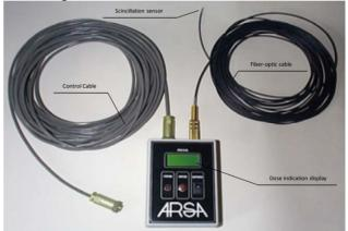
Figure 2: Fiber-optic monitor-dosimeter, combined with ARSA control panel.
