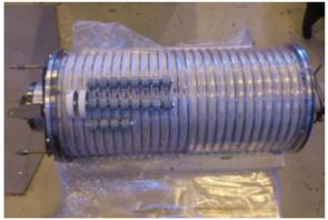
Figure 5: Modified accelerating tube.
