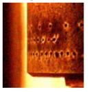
Figure 5: Graphite target of the laser ion source. The lower compact row of spent emitting spots stands for the present, optimised operation.
