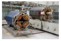
Figure 14: Wide-aperture quadrupole lenses of the new Proton Radiographic Facility at IHEP.
