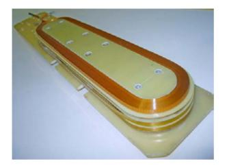
Figure 13: Four-layer racetrack coil from HTS-2G tape.
