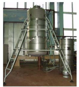
Figure 8: Cryogenic helium vacuum heat exchanger (10g/s helium flow, 300-2 K temperature range).
