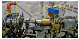
Figure 5: Diagnostic beam line. 1 - RF gun; 2 - focusing solenoid; 3 - first beam current sensor; 4 – beam steerer; 5 - vacuum chamber of 160 mm in diameter; 6 - solenoid; 7 - vacuum ion pump; 8 - movable target; 9 - the second beam current sensor; 10 - rotating beam steerer; 11 - 30 kW beam dump; 12 - lead radiation shielding.
