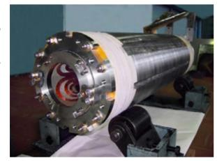
Figure 5: SIS300 fast cycling quadrupole prototype.
