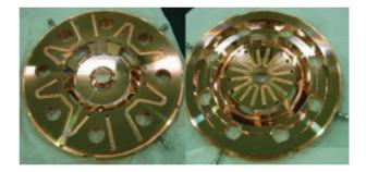
Figure 6: ACS half cells for J-PARC linac
