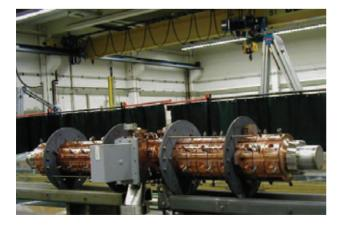
Figure 8: CDS booster cavity for PITZ
