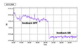
Figure 9: The VEPP-4M guide field stabilization.
