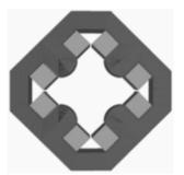
Figure 2: General view of the quadrupole magnet.
