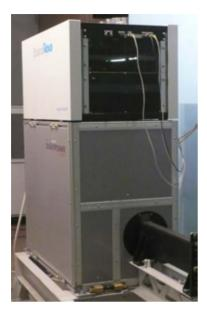
Figure 4: Accelerator for cargo inspection.. Table 2: Cargo inspection accelerator parameters.
