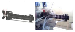
Figure 4: Target device for production of C-11.
