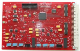
Figure 3: Printed circuit board of the quench detector
