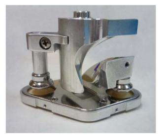
Figure 4: The electrodes of the spiral inflector.
