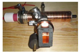
Figure 1: Accelerating system.
