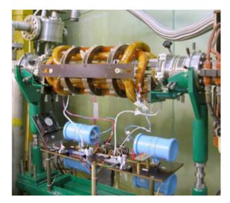
Figure 1: Windings assembly with the capacitor bank.
