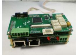
Figure 5: The accelerator controller without a box.
