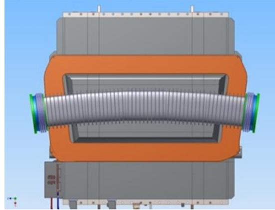
Figure 4: Half of the dipole yoke with the 2 mm thick elliptical vacuum chamber with ribs.
