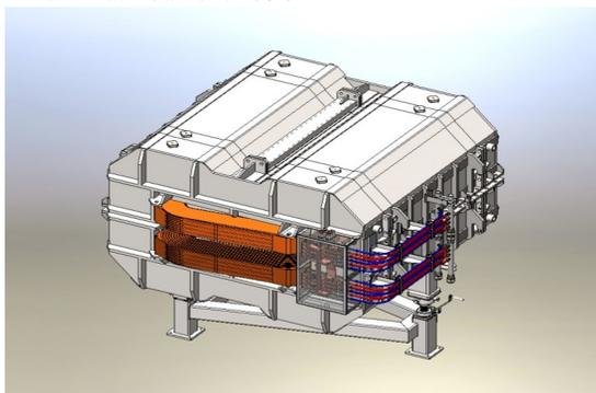
Figure 3: 3d model of the CR dipole magnet.
