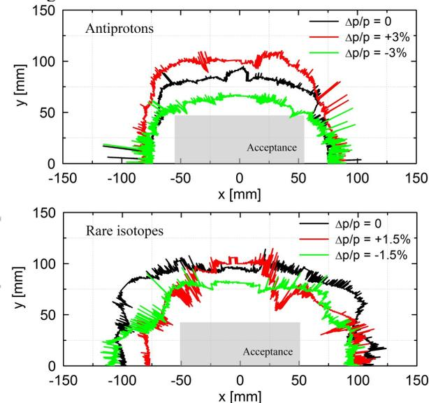
Figure 8: MAD-X dynamic aperture simulation results.
