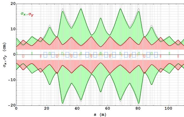
Figure 7: Beam size along one half of the ring.
