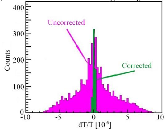
Figure 9: Effect of sextupole and octupole corrections on TOF distribution.
