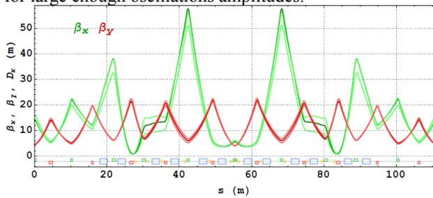
Figure 6: Lattice functions for on-energy particle (dark) and off-energy particles (light).
