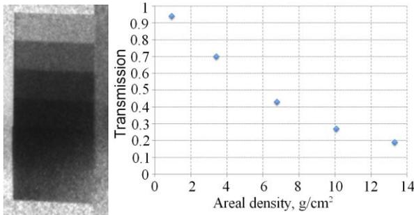
Figure 2: Proton radiography image of tantalum steps wedge and transmission/areal density diagram.
