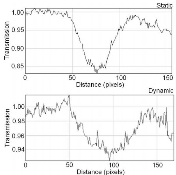
Figure 6: Profile of static and dynamic images of Ta wire.
