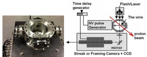
Figure 4: Photo and scheme of underwater electrical wire explosion target.
