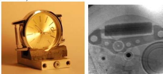
Figure 3: Photo and proton radiography image of quartz watch.
