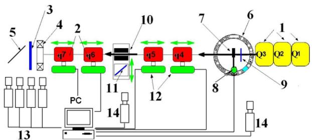
Figure 1: Photo and scheme of PRIOR proton microscope. 1- electromagnetic quadrupoles (matching section), 2- quadrupole lenses on permanent magnets PMQ (magnification section), 3-scintillator, 4- fast current transformer, 5- mylar foil mirror, 6- vacuum or water target chamber, 7- target, 8- target manipulator, 9- beam position/profile monitor (Bicron scintillator), 10- collimators, 11- beam position monitor, 12- linear actuators, 13- fast CCD cameras, 14- CCD cameras for beam tune
