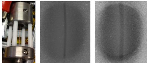
Figure 5: Photo and proton radiography images of tantalum wire.
