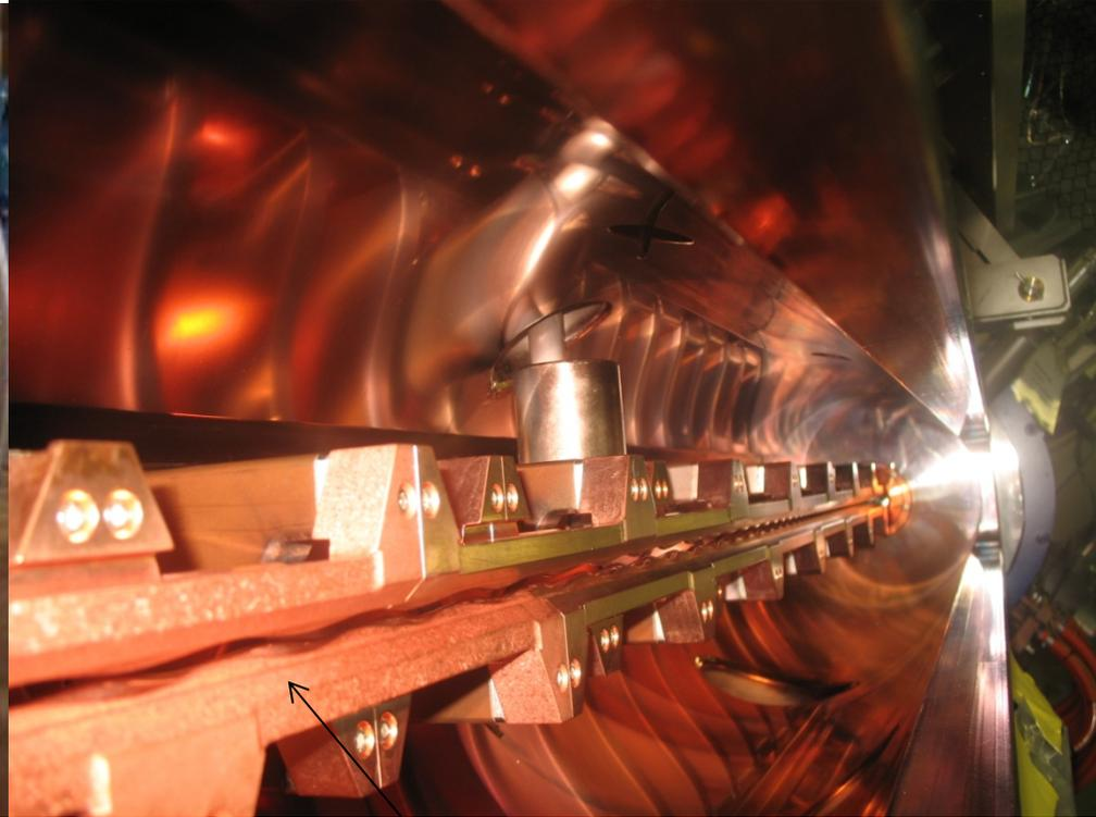
**Acceleration and bunching is performed by sophisticated modulation of the rods**
