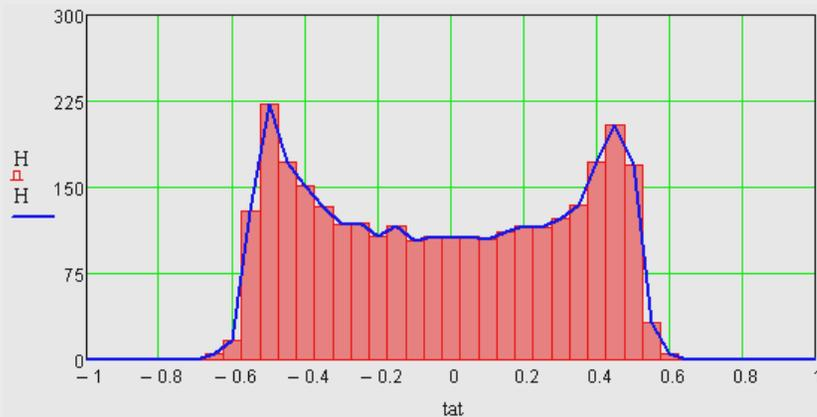
Histogram of the output beam current density
