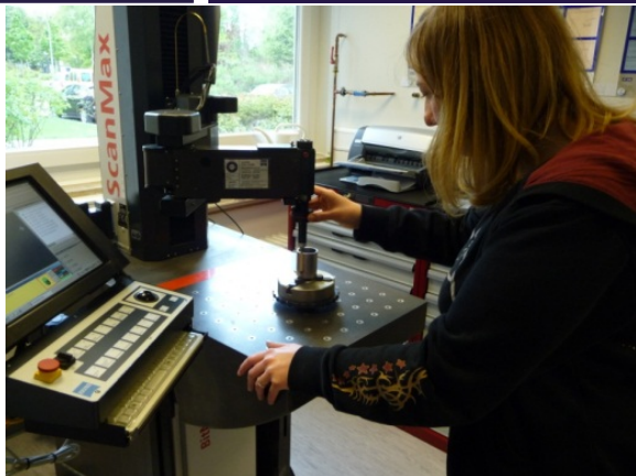
Equipment for tactile 3D dimension measurement
