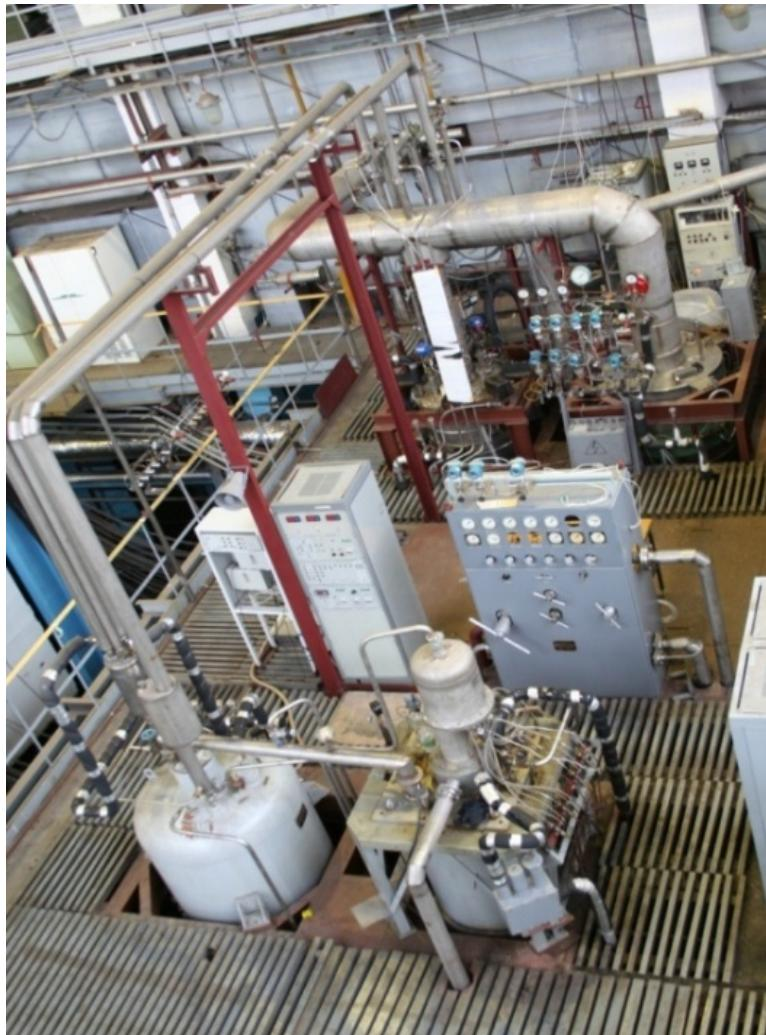
Cryogenic helium vacuum heat exchanger (10g/s helium flow, 300-2 K temperature range)
