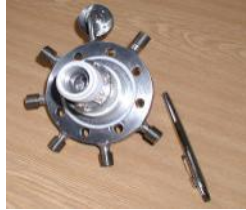
wet turboexpander (300 000 turns/min)
