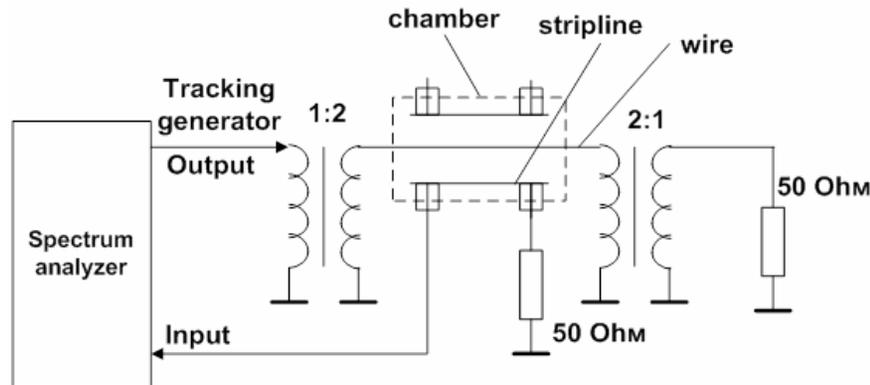
Measured sensitivity @ 500 MHz is about 9 V/A;
