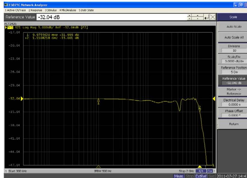
The upper cut off frequency @ -3 dB is 1.1108 GHz.
