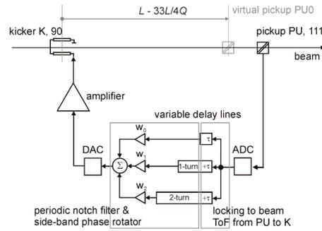
Figure 11: Updated layout of the wide-band feedback.
