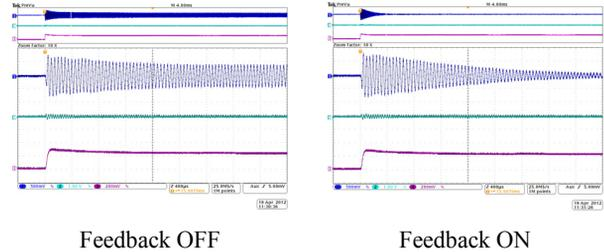
Figure 12: Damping of radial oscillations at injection (upper traces). Lower trace is beam intensity (DCCT).
