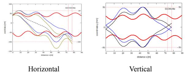
Figure 13: Waiting beam envelope ( $\delta p/p_0 = \pm 3 \cdot 10^{-3}$ ) and representative traces for extracted fraction (ionization loss  $\Delta p/p_0 = -0.69\%$  and  $\pm 2\sigma_{\text{MCS}}$  in slope over IT#28).
