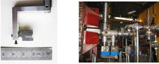
Figure 14: Energy-degrader inner target IT#28 (beryllium, thickness 4.0 mm, height 10 mm) for carbon beam and the IT outer assembly at SS#28.
