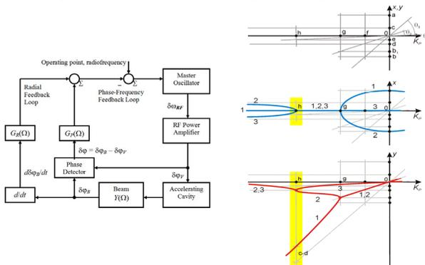
Figure 9: Block diagram of RF control in the U70. Figure 10: Characteristic equation root map.
