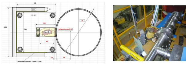
Figure 15: Deflecting septum magnet SM#34 (80 mrad, 0.42 T, 1.3 m, 80×40 mm<sup>2</sup> (h×v)).
