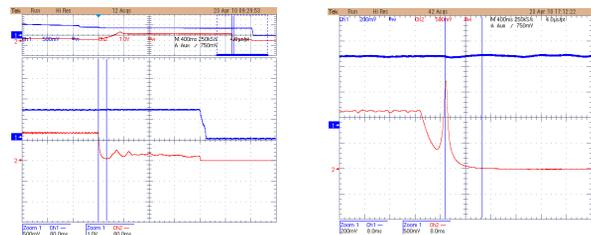
Figure 19: Suppression of self-bunching at 50 GeV flattop and  $7 \cdot 10^{11}$  ppp with RF gymnastics. Upper (blue) trace is beam intensity (DCCT). Lower (red) trace is beam peak current signal.
