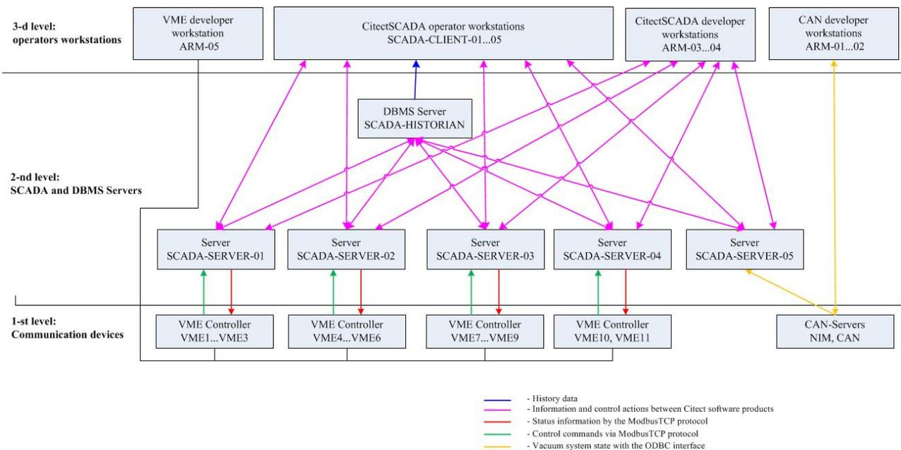
Fig.3. Functional structure of the TS.
