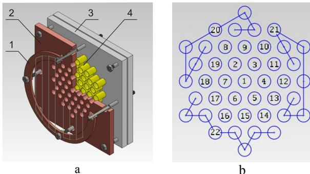
Fig. 3. a) Beam detector: 1 - suppressing grid, 2 - copper plate, 3 - insulating plates, 4 - Faraday cups. b) Numbering of detector channels.
