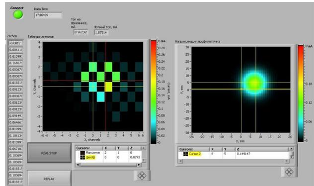
Fig. 4. User interface of the beam registration program.
