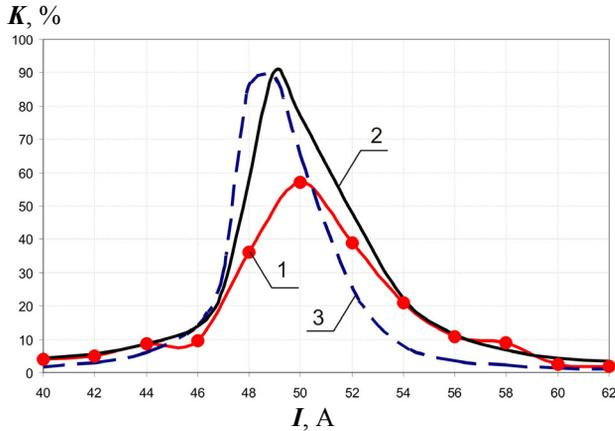
Fig. 6. The dependence of the percentage  $K$  of beam current in the axial region with a diameter of 5 mm on the current of magnetic focusing lenses  $I$ : 1 - measured, 2 - calculated at  $T = 0$  eV, 3 - calculated at  $T = 10$  eV.
