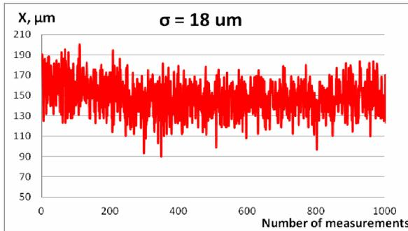
Fig.7. Results of horizontal beam position measurements for number of particles per bunch  $\sim 0.5 \times 10^{10}$ .
