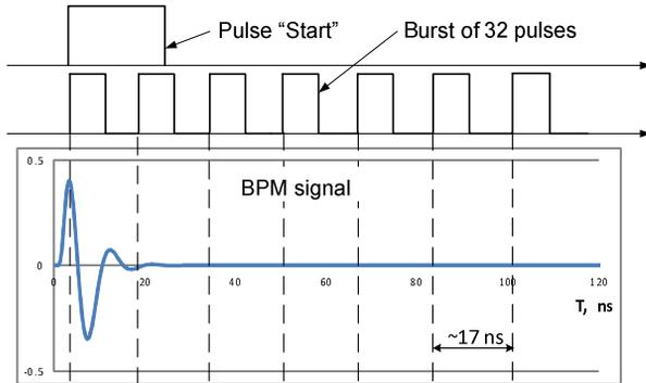
Fig.3. A time diagram of the timing circuit.
