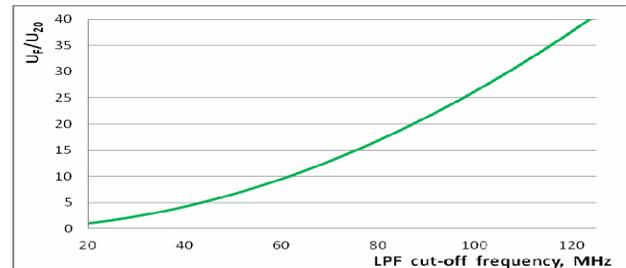
Fig.1. Calculated dependence of the relative signal amplitude in the LPF output  $U_F / U_{20}$  on the  $F_{LPF}$ .
