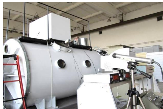
Figure 4: Equipment for electron-beam welding.
