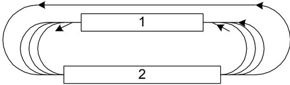
Figure 1: Scheme of ERL with two linacs.
