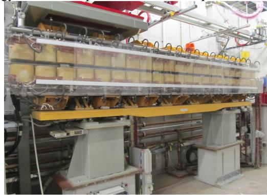
Figure 2: FLASH far infrared undulator constructed by JINR.
