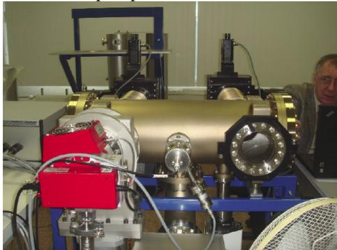
Figure 1: XFEL SASE1&SASE2 MCP detector.
