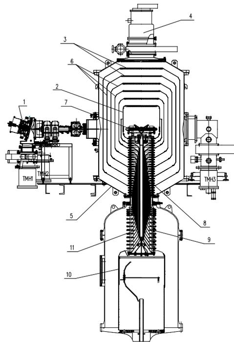
Fig. 1. Scheme of the VITA facility. 1 – ion source (H); 2 – high voltage electrode; 3 – electrode shutters; 4 – cryo pump; 5 – accelerator vacuum volume; 6 – intermediate electrodes; 7 – stripping target; 8 – feedthrough insulator (vacuum part); 9 – feedthrough insulator (gas part); 10 – high voltage source; 11 – coaxial feeding tubes.
