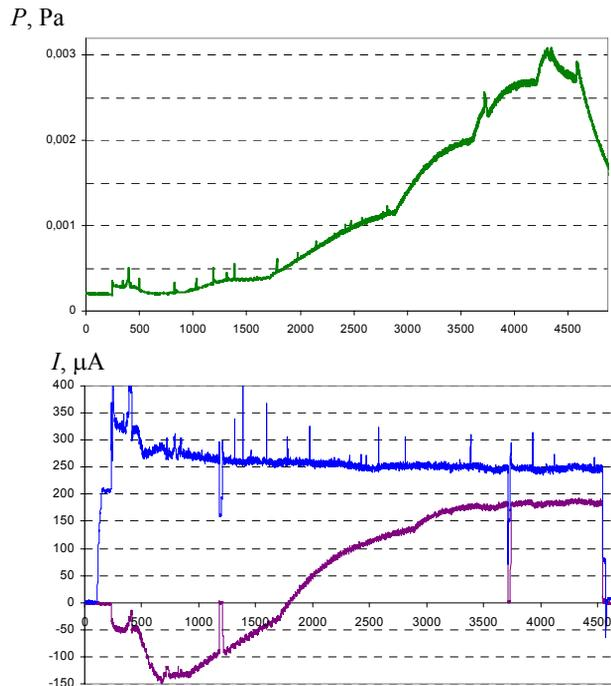
Fig. 4. Time dependence of the residual gas pressure P (a), the accelerator current  $I_{acc}$  (b, upper line) and beam collector current  $I_{out}$  (b, bottom line).
