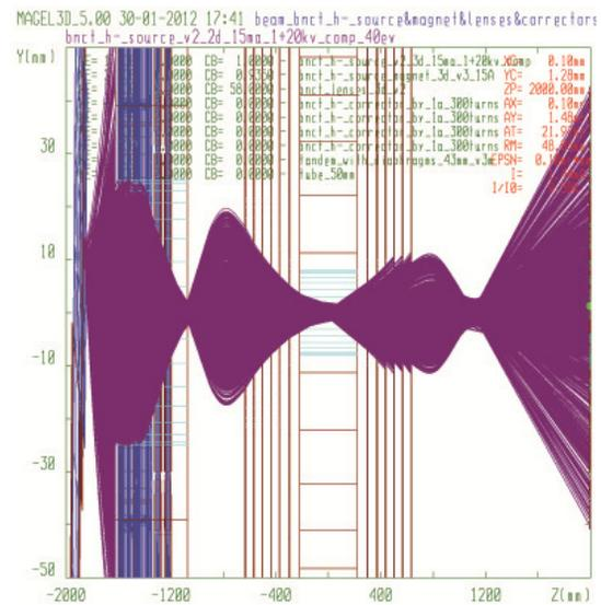
Fig. 6. Calculated trajectories of negative ions in the tandem-accelerator (ion source is located at the left side,  $Z=0$  corresponds to the middle of the stripping target and the output beam collector is located at the right side at the point  $Z = 1500 \text{ mm}$ ).
