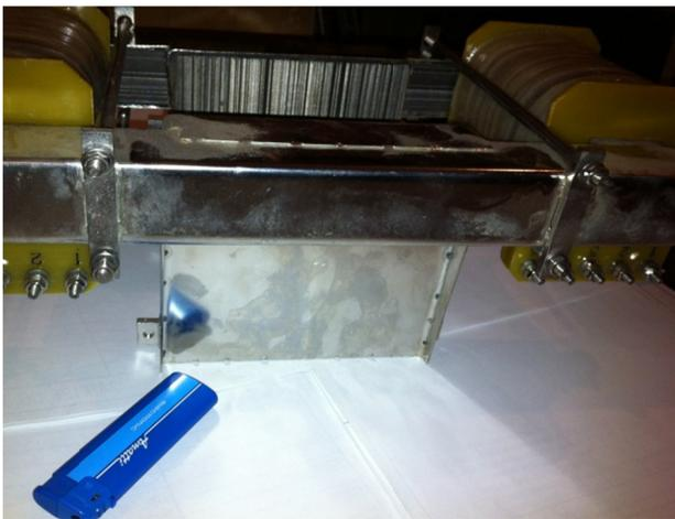
Figure 4. LF scanner coils.
