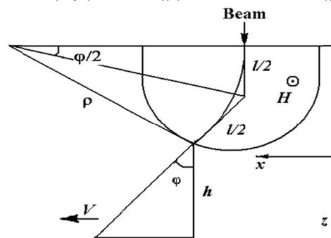
$$Y_V = \frac{V(\varphi)}{V(\varphi=0)} = \frac{\cos^2(\varphi/2)}{\cos^2(\varphi)}; Y_D = \frac{\cos(\varphi)}{\cos^2(\varphi/2)}$$
