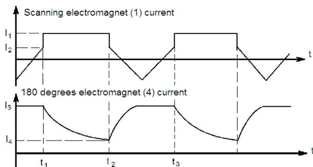
Fig.2. Electromagnets currents.
