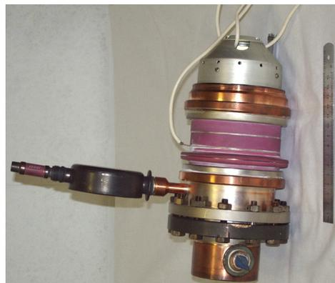
Figure 2: Electron gun after manufacturing.
