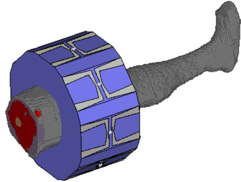
Fig. 1: Voxel model of leg inside phase array.
