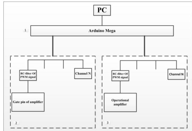
Fig.3: Control system schematic layout.
