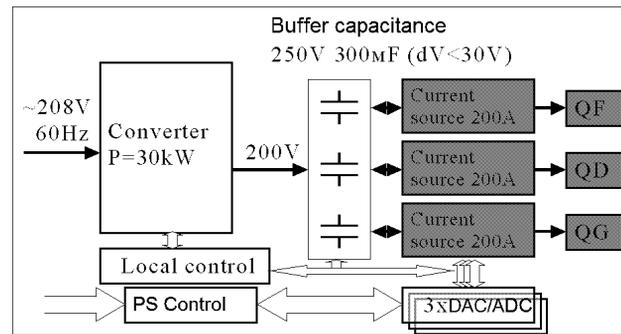
Fig. 2. Power source block diagram.
