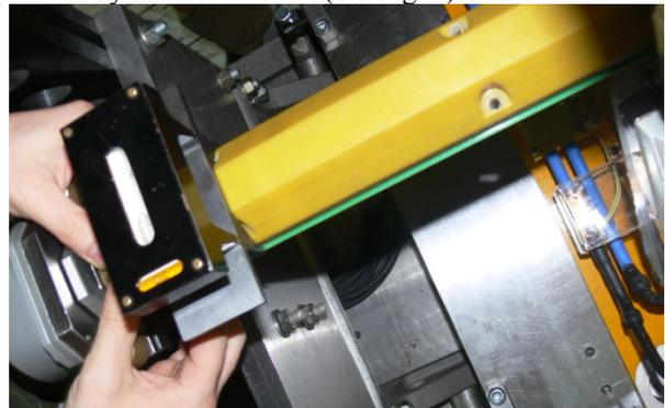
Figure 6. The shaft levelling.
