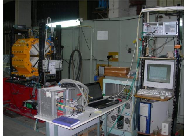
Figure 1. Magnetic measurement stand.
