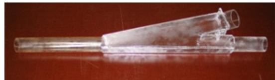
Figure 2: Glass vacuum chamber
