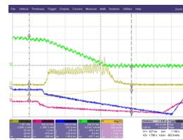
Traces from top to bottom: (1) circulating C beam intensity; (2) slow spill (a saturated signal); (3, 4) coil currents for closed-orbit bumps near IT#28 and SM#34, resp.
