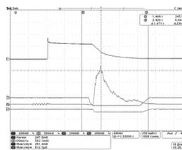
Traces from top to bottom: (1) circulating C beam intensity; (2) slow spill (a proportional signal); (3, 4) coil currents for steady closed-orbit bumps near IT#28 and SM#34, resp.
