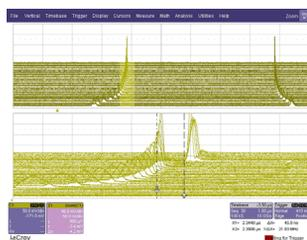
Scan period is 5000 turns. Scans are locked to the RF phase, and apparent jump of the bunch is, thus, virtual.
