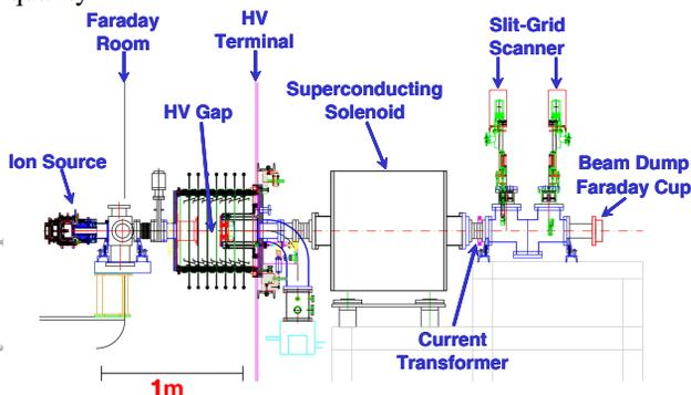
Figure 2: Injection scheme for high current uranium production
