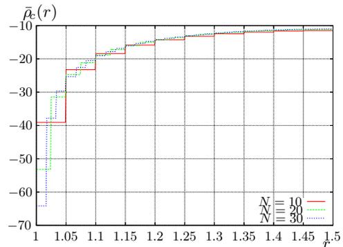
Figure 2: Space charge density, cylindrical diode, one-dimensional case
