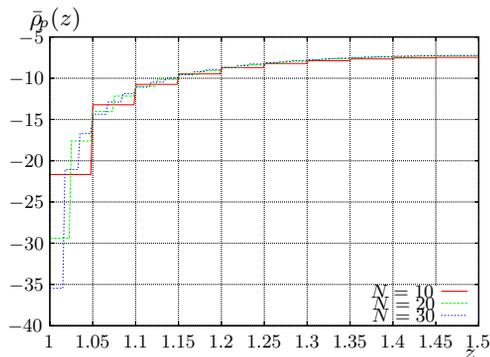
Figure 1: Space charge density, plane diode, one-dimensional case
