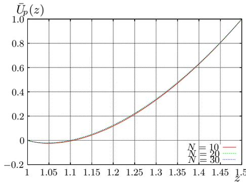
Figure 3: Potential distribution, plane diode, one-dimensional case
