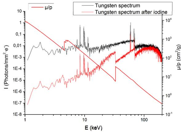
Fig. 1. Spectrum of X-ray tube with tungsten anode, spectrum after iodine contrast agent and iodine mass attenuation coefficient.
