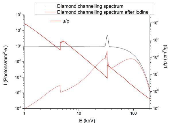
Fig. 2. Spectrum of channelling X-ray obtained from diamond crystal with 21 MeV electron beam, spectrum after iodine contrast agent and iodine mass attenuation coefficient.
